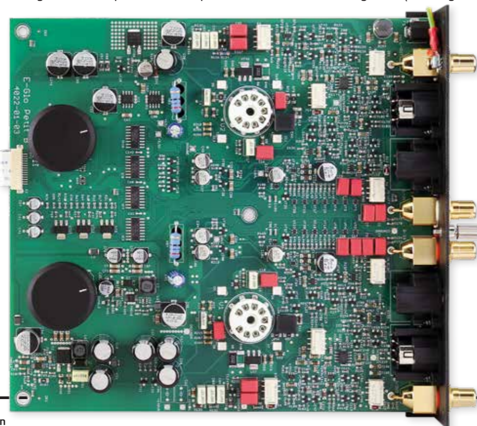
RIGHT: Powered by an outboard 18V DC PSU, the E-Glo Petit B combines a discrete, low-noise J-FET front-end [far right] with a two-stage ECC83S triode-based RIAA preamp [centre]. Gain and loading options are switched by logic [left]
